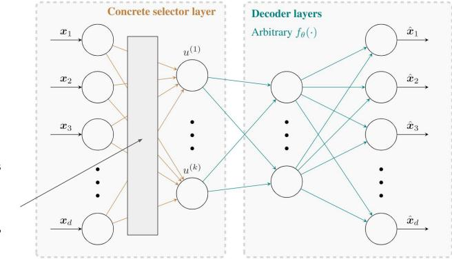
Replace the weights of the encoder with parameters of a **Concrete Random Variable** (Maddison, 2016)
