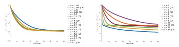
Figure: On sparse logistic regression, the plots are gradient ADMM and the differential inclusion when  $\rho=10$ , first plot is for different  $\alpha$  from  $2^{-3}$  to 2 when c=10, second plot is for different c from 1 to 32 when  $\alpha=1.6$
