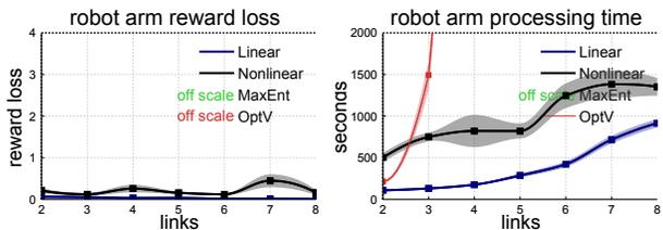
Figure 6. Reward loss and processing time with increasing numbers of robot arm links  $n$ , corresponding to state spaces with  $2n$  dimensions. Our methods efficiently learn good rewards even as the dimensionality is increased.
