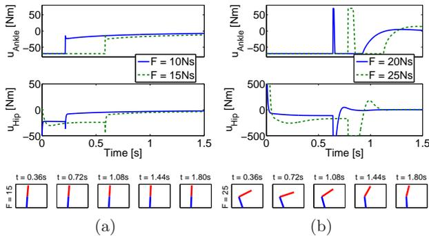
Figure 6. Learned solutions for the 2-link balancing problem for (a)  $F = 10\text{Ns}$  and  $F = 15\text{Ns}$  (ankle strategy) (b)  $F = 20\text{Ns}$  and  $F = 25\text{Ns}$  (ankle-hip strategy). The sketches below illustrate the temporal course of the balancing movement for the ankle strategy (a) and the ankle-hip strategy (b)
